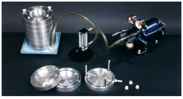
Figure 5. A 2-stage (foreground) and a 6-stage Andersen sampler. A 6-stage Andersen sampler properly connected to a flowmeter and a vacuum pump (background).
